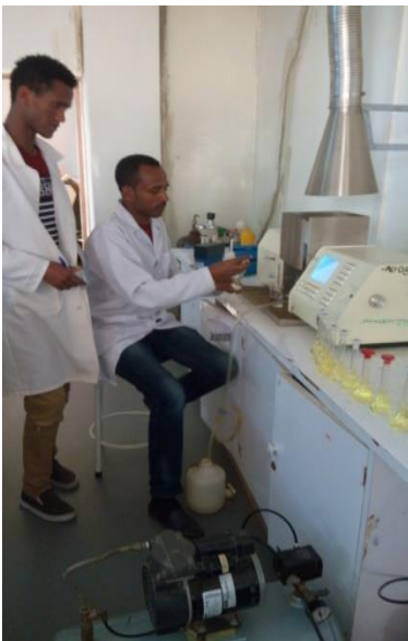
During determination of heavy metals (Pb, Cd, and Cr) by an instrument called Atomic Absorption Spectrophotometry (AAS) at HU, central laboratory
