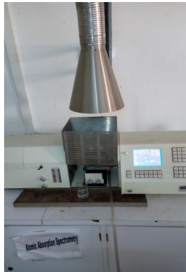
During determination of heavy metals (Pb, Cd, and Cr) by an instrument called Atomic Absorption Spectrophotometry (AAS) at HU, central laboratory
