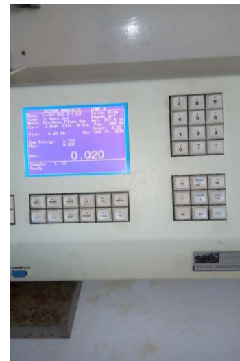
During determination of heavy metals (Pb, Cd, and Cr) by an instrument called Atomic Absorption Spectrophotometry (AAS) at HU, central laboratory
