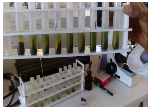
5 ml of sediments after centrifugation
