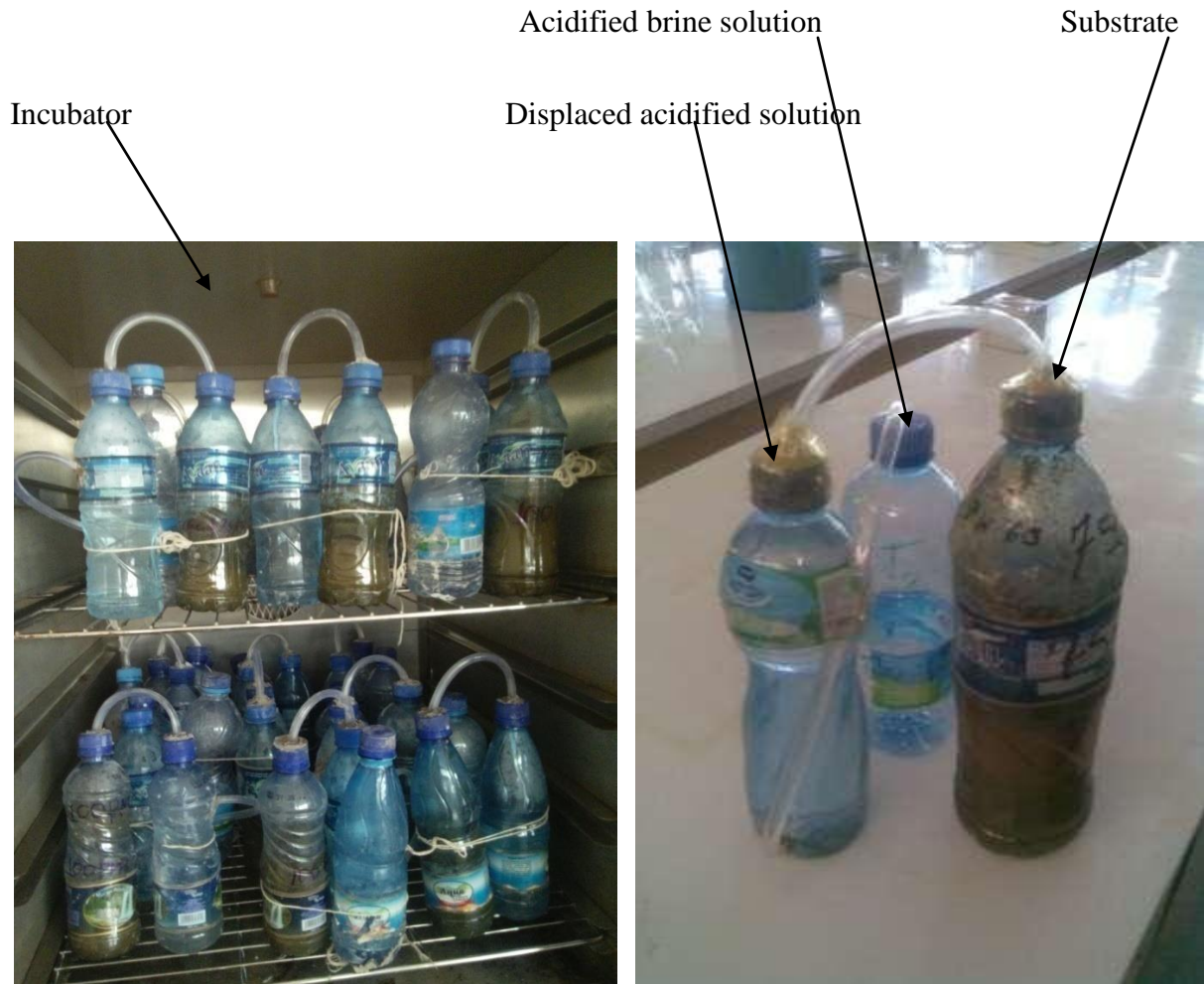
Figure 1. Configuration and setup of the digester
