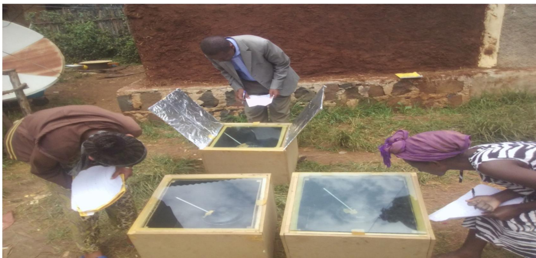
Figure3. Temperature and time measurements done simultaneously for three boxes.
