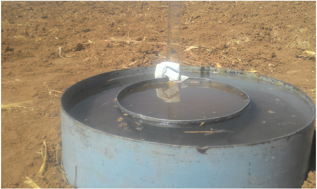
Appendix Figure 3: Soil Infiltration Capacity Test of Study Area
