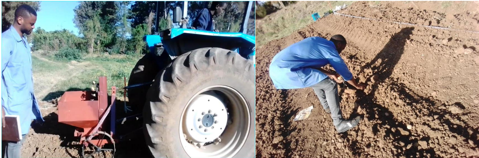
Appendix Figure 4: Testing prototype tractor mounted potato planter and measuring the spacing between tubers
