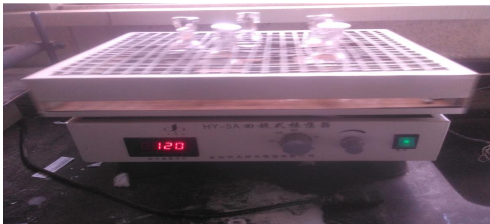
Rotary shaker for proper mixing of phosphate and sandstone
