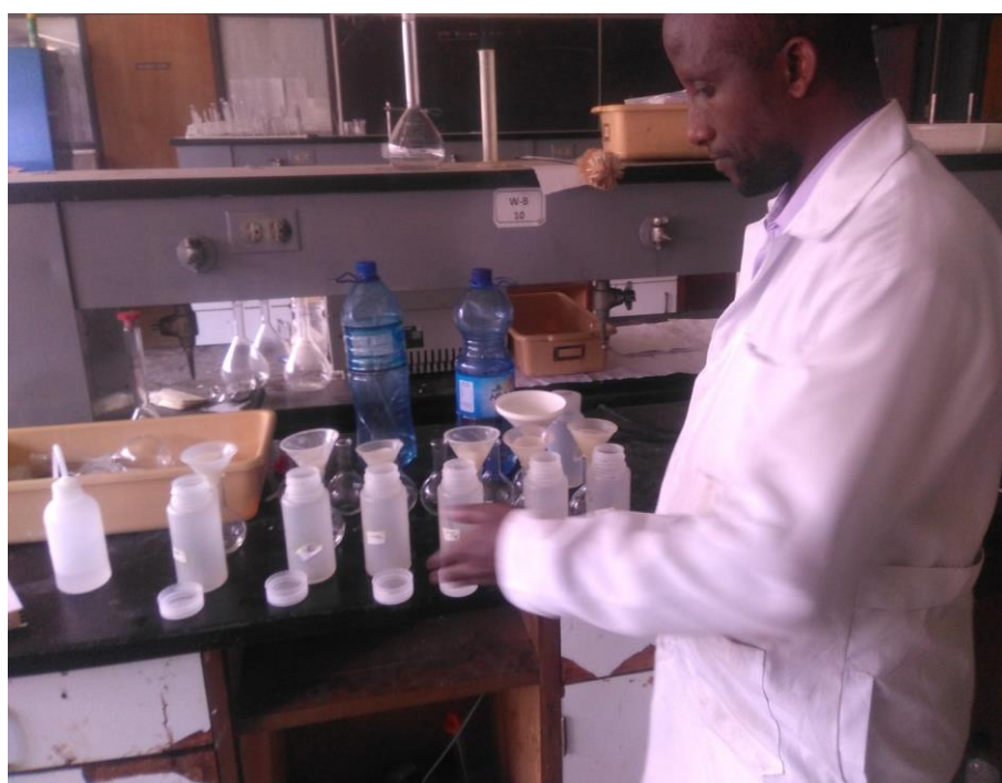
Preparation of residual phosphate through filtration for spectrometric determination
