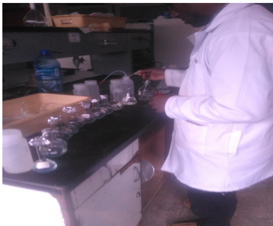
Color development during addition of reagent to residual phosphate
