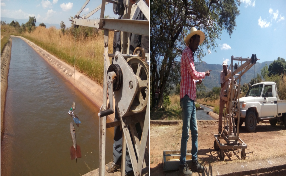
Figure 3. : Data collecting byUS D-74 Suspended Sediment Sampler.
