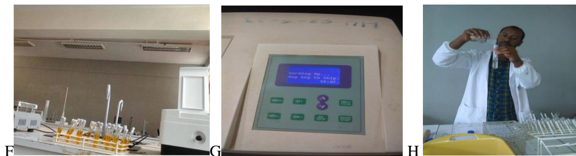
Figure 6.sample ready to read reducing sugar at 540nm and cell density at 540nm by spectrophometre.
