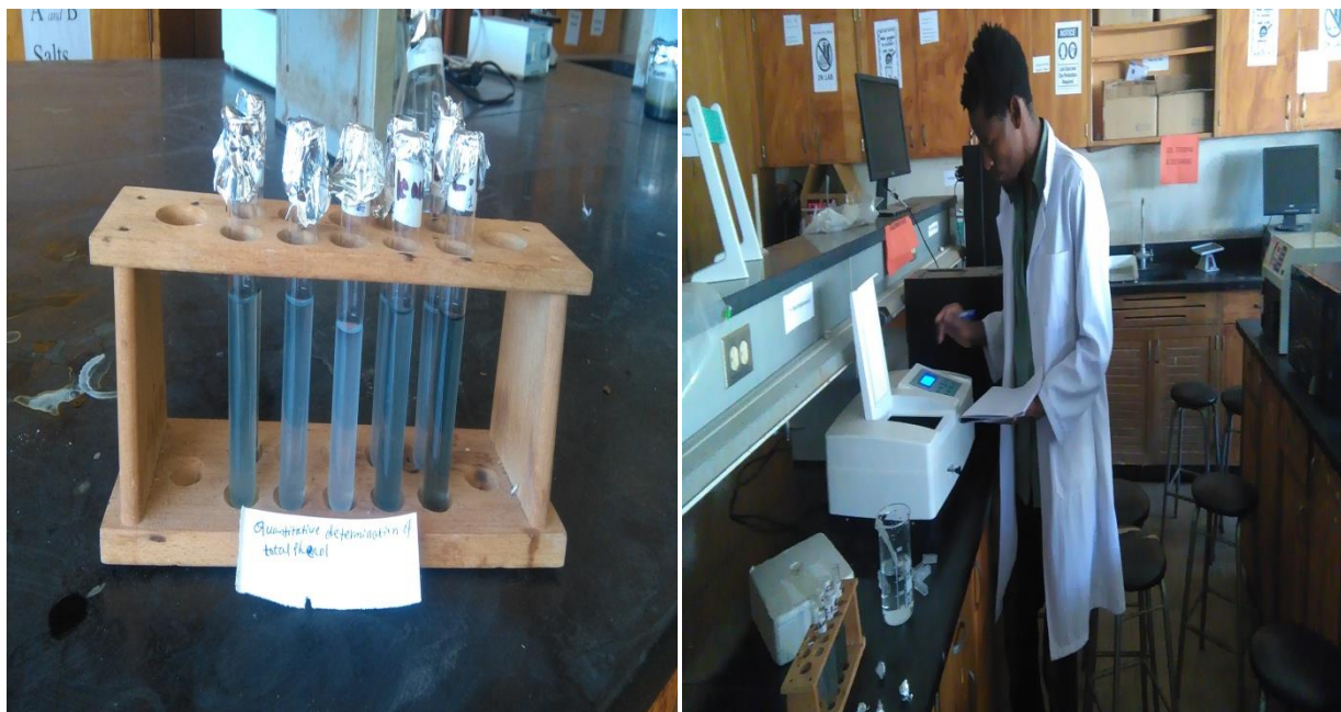
Figure 5: Phenol Content Determination by using UV- Spectrophotometer
