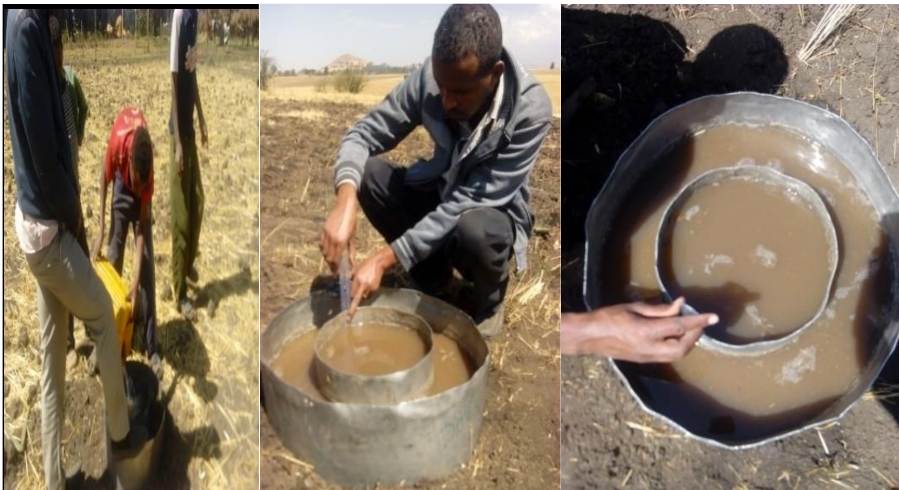
Appendix Figure 4.. Infiltration Measurement of Selected Plots
