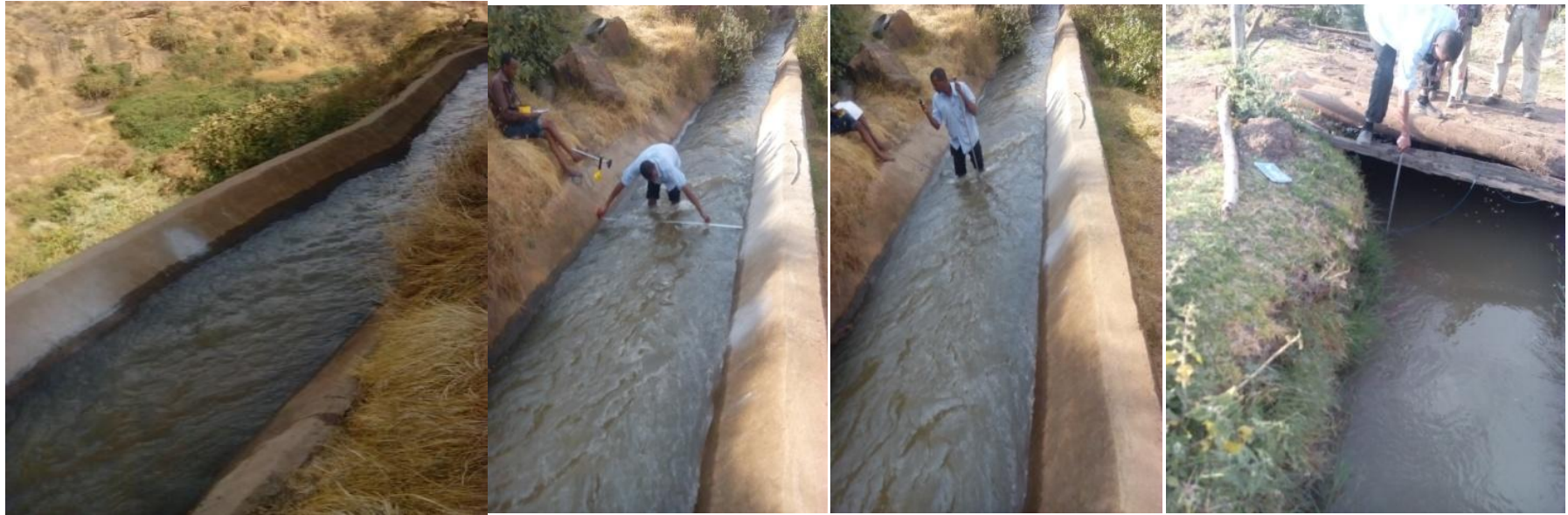
Appendix Figure 1. Discharge Measurement by Current Meter at Diversion head and Different Segments
