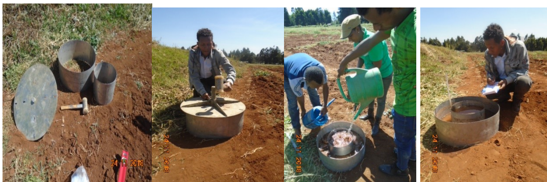
Appendix figure 3. Photography taken during measuring of the infiltrations rate by digital camera
