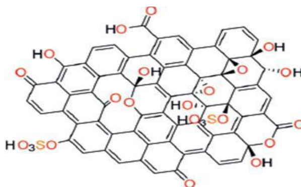
Figure 2. Structure of graphite oxide with some functional groups
